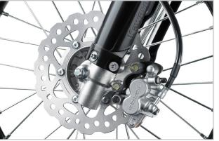
Large-diameter 220 mm front brake gripped by a dualpiston caliper is complemented by a 184 mm disc and single-piston caliper at the rear.
